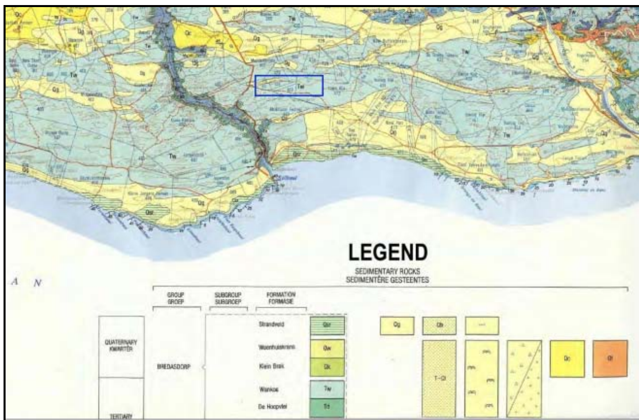
Figure 5. Geological map of the Still Bay district with the area of focus for the Lunsklip Wind Farm enclosed by a blue rectangle. The area is underlain by sediments of the Wankoe Formation, Bredasdorp Group with a covering of Quaternary Regic Sands in many places (Source: 1:250 00 Geological Series Map – Riversdale).
