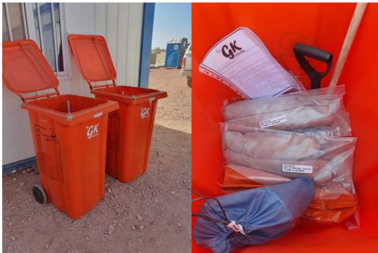
Figure 17: Hydrocarbon Spill Kits must be in place within the site camp and in the field within 500m of any drilling or ramming activity.
