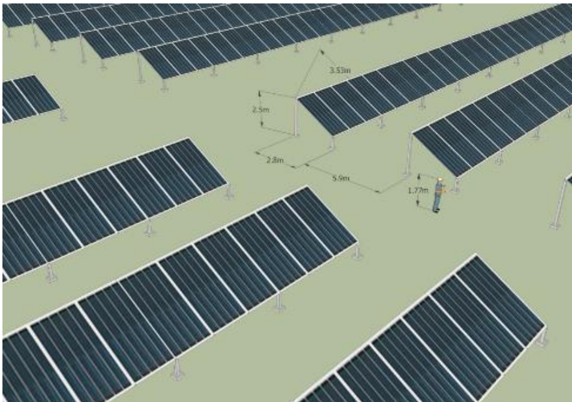
Figure 24: Photographic 3D model used to inform the photomontages showing 2.5m height versus 4.3m height.
