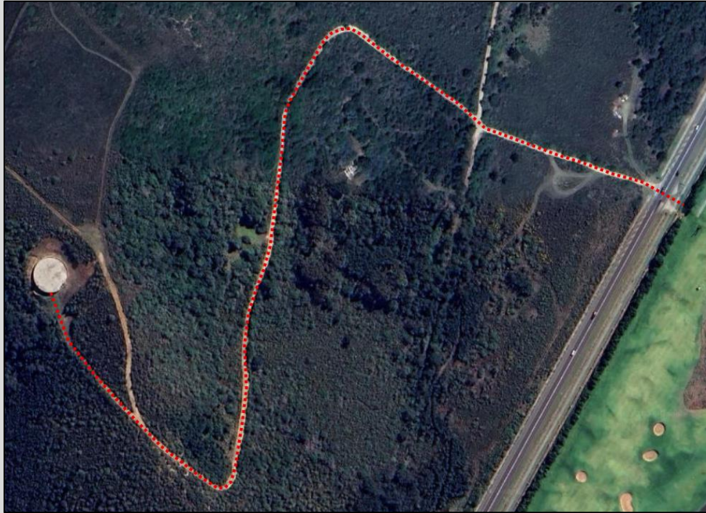
Figure 7: Preferred pipeline route from Goose Valley Reservoir to existing distribution main in N2 road reserve.
