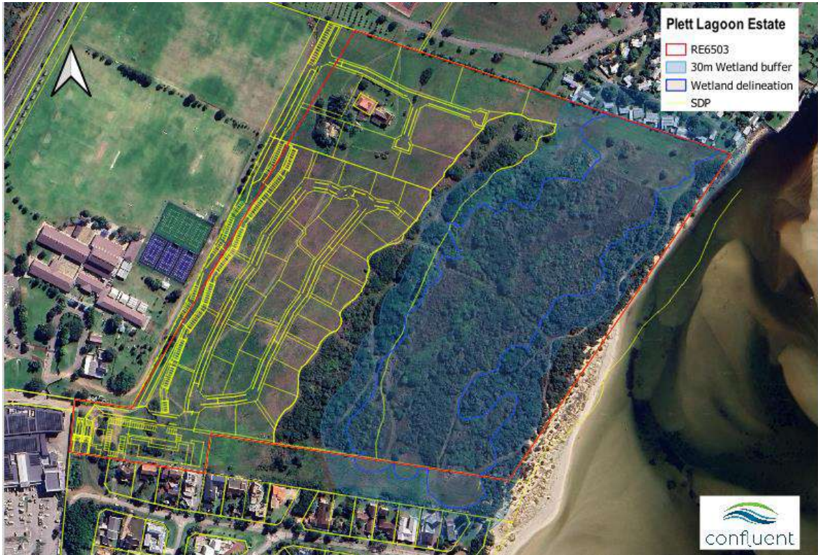
Figure 3: Site Development Plan, Delineated wetland and 30 m wetland buffer on the development site for Plett Lagoon Estate, RE/6503, Plettenberg Bay. **Note: The property boundary for RE/6503 is incorrect on Cape Farm Mapper and includes the piece of land adjacent to the school grounds to the northwest as per Title Deed T 98661/1996.
