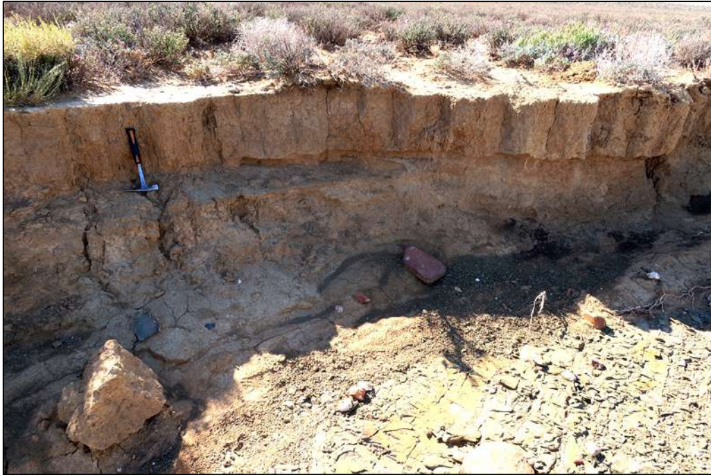
Figure 28: Section through the younger sandy alluvium with sparse dispersed gravel clasts overlying Tierberg Formation bedrocks, banks of the Klein-Droëlaagte on Hoek Doornen 172 (Hammer = 30 cm).
