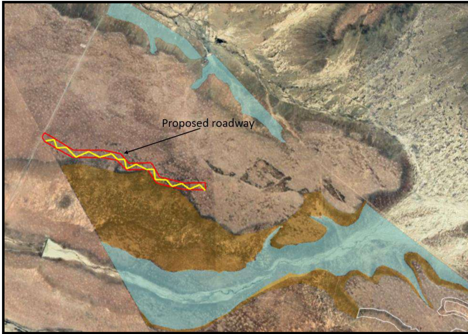
Figure 3. Map image detailing the position of the proposed access road relative to the sensitive areas within the site.
