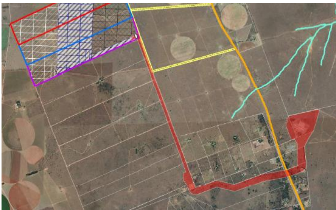
Figure 3: Proposed powerline corridor (red) between the Houthaalboomen North Collector substation / switching station and the Watershed MTS.
