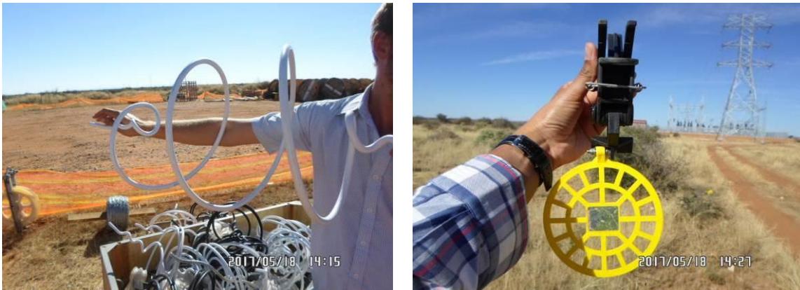
Figure 19: Examples of bird flight diverters to be used on the power lines: Double loop bird flight diverter (left) and Viper live bird flapper (right).
