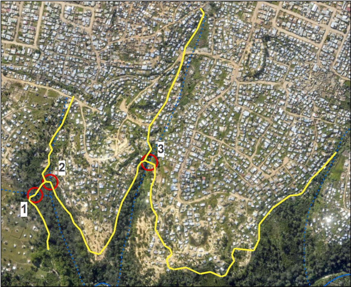
Figure 17: Location of three main tributary crossings (Red Circles) along the new proposed sewer pipeline route.
