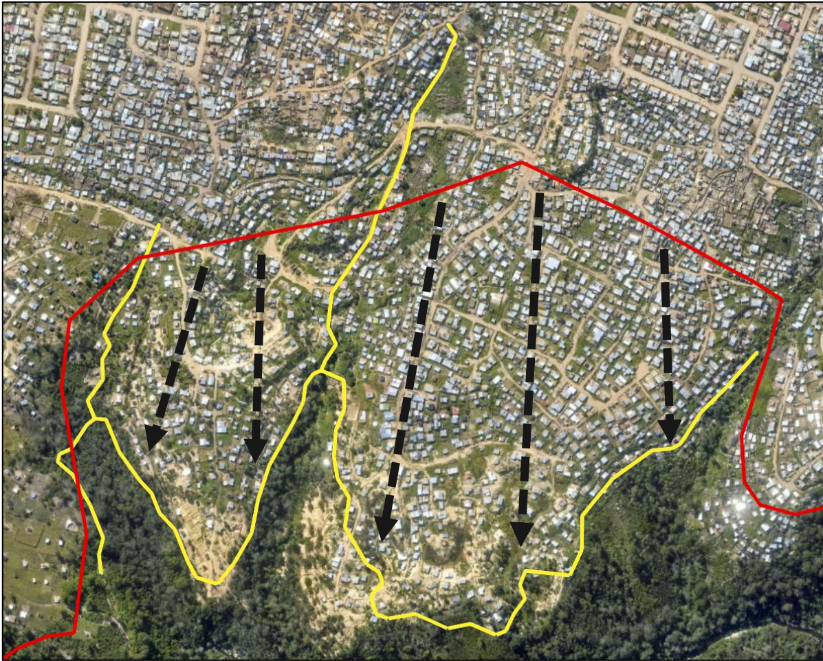
Figure 16: Proposed pipeline route (Yellow Line) around the southern border of the old 'All Brick' brickworks. Original approved pipeline route (Red Line).
