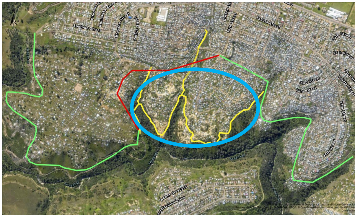
Figure 1: Green = Approved pipeline route ( already constructed ). Red = Approved pipeline route (not yet constructed). Yellow = Proposed amended pipeline route (to be constructed still).
