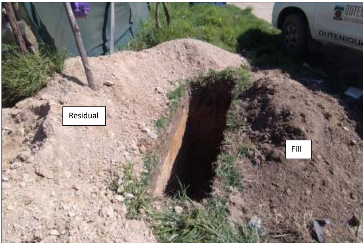
Figure 16: Typical soil types exposed at TP5
