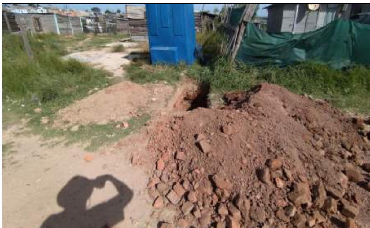
Figure 15: Brick rubble fill encountered at TP1
