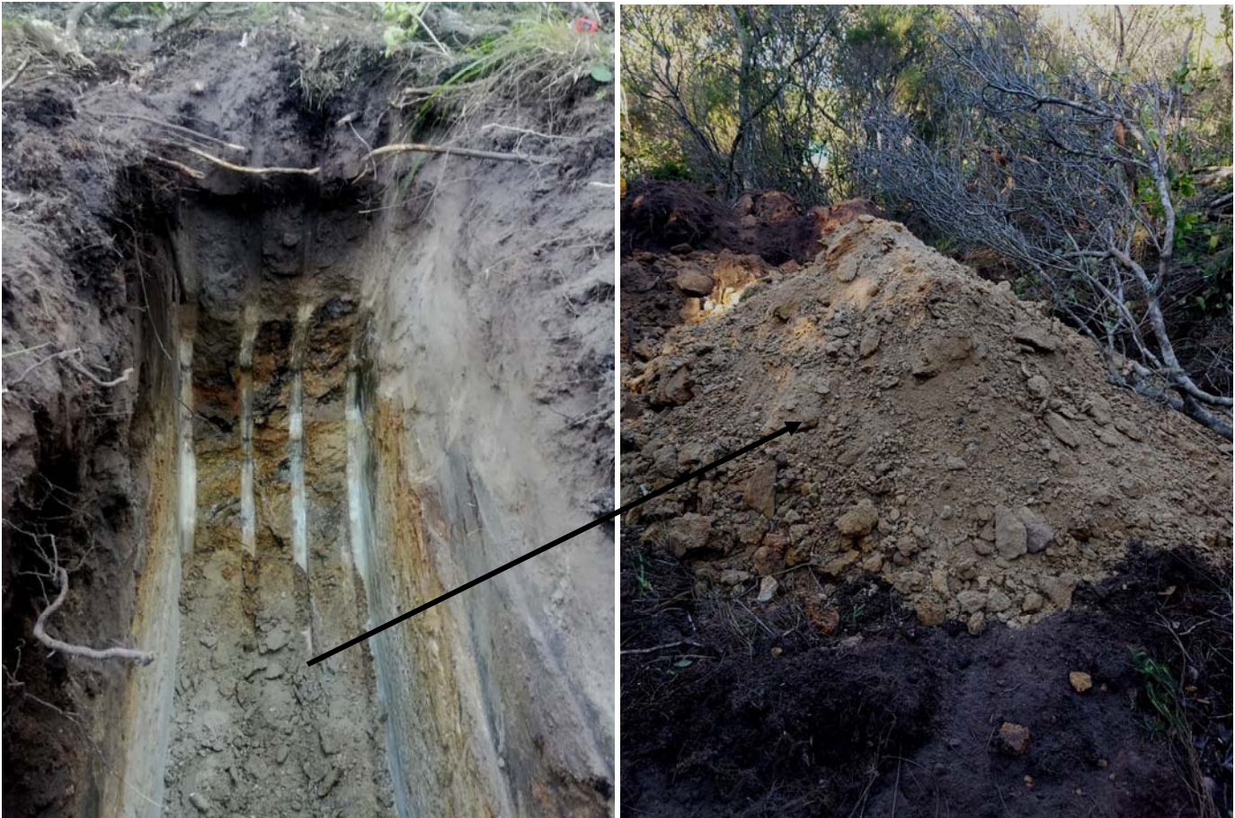
Fig 2: Typical soil profile and weathered granite gravel excavated from test pits
