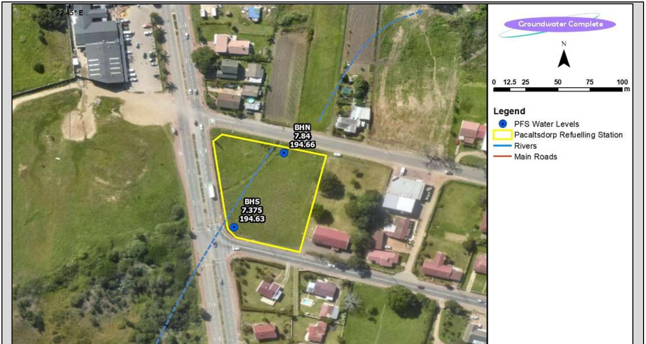
Figure 7: Water level depths below surface and elevation recorded during the hydrocensus (Groundwater Complete, 2025).
