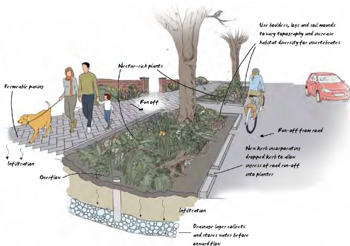
Figure 11: An image illustrating some ideas for more sustainable urban drainage systems (SuDS), as illustrated in the SuDS handbook (Graham, 2016).
