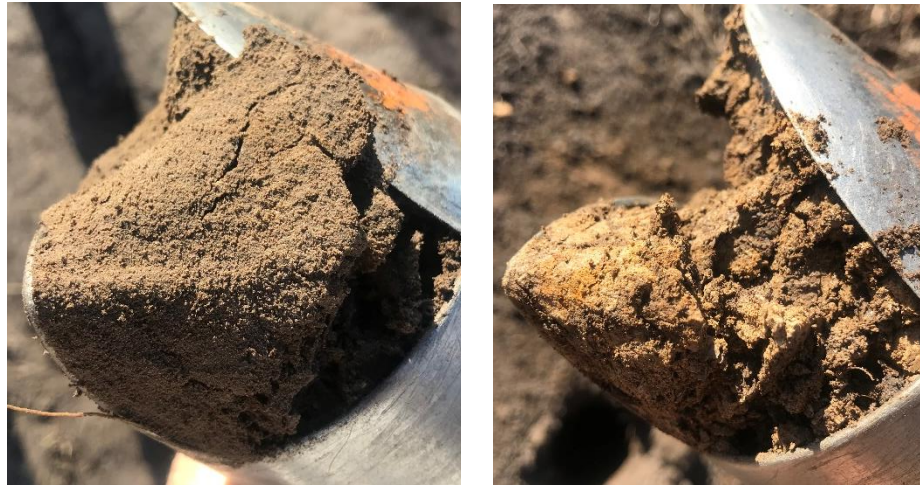
Figure 12. Example of augered soil down the slope towards Camphersdrift wetland showing soil with no wetland indicators (left) compared to soils with indicators of temporary wetness (right).
