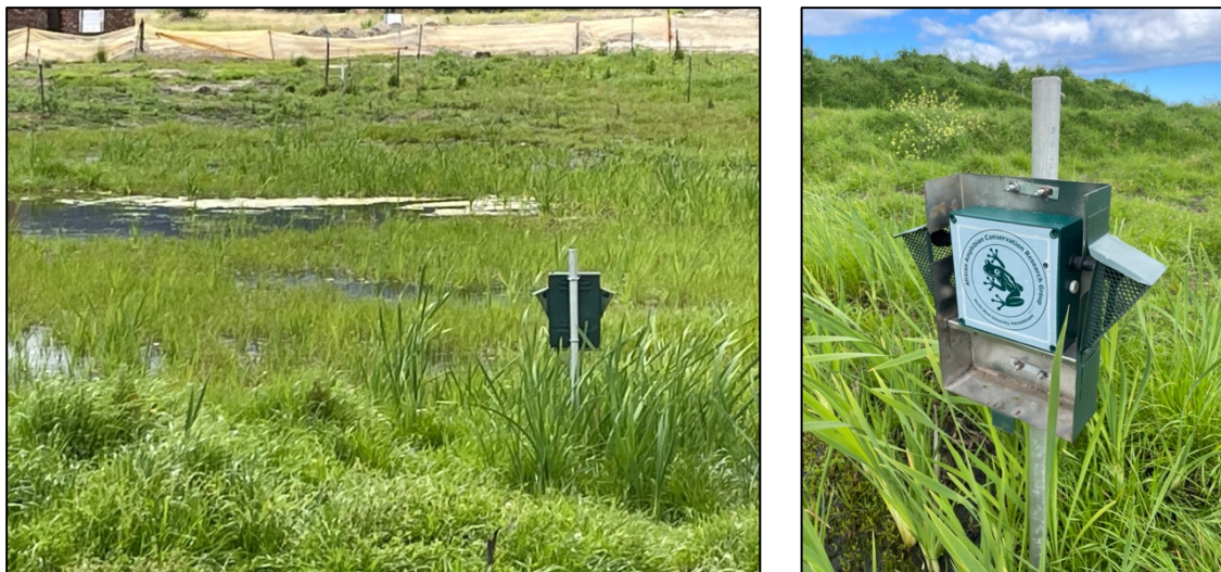
Figure 2: Song Meter® SM2+ within protective housing, mounted against single post planted within the wetland site
