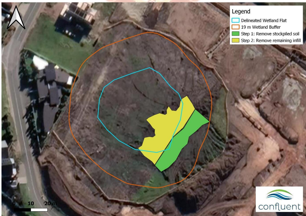
Figure 3: Map showing Step 1 and Step 2 soil to be removed from the Wetland Flat and buffer area
