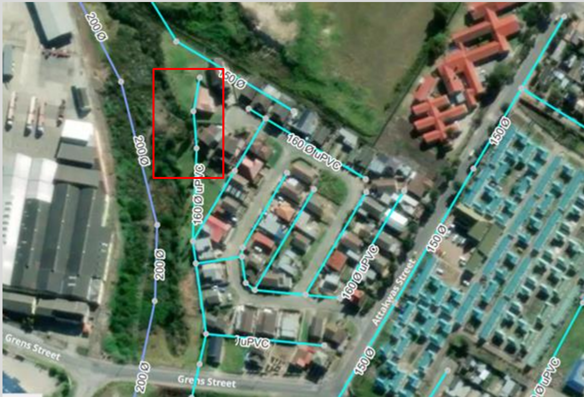
Figure 2: Figure indicating the approximate sewer lines along the watercourse in blue line (200 & 160).
