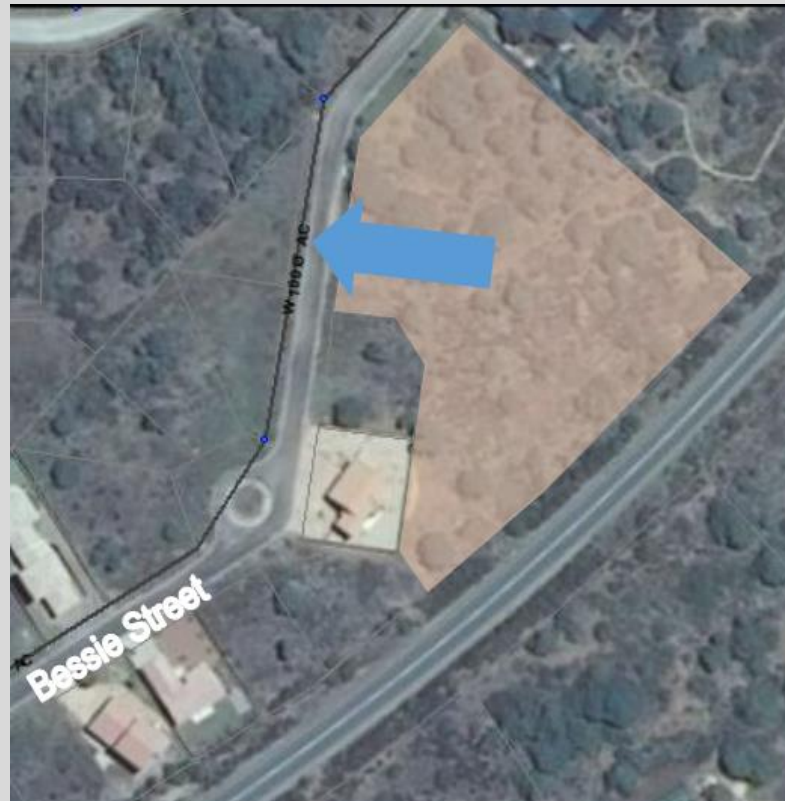
Figure 5: Existing Municipal 100mm water line for connection purposes (Element Engineers).
