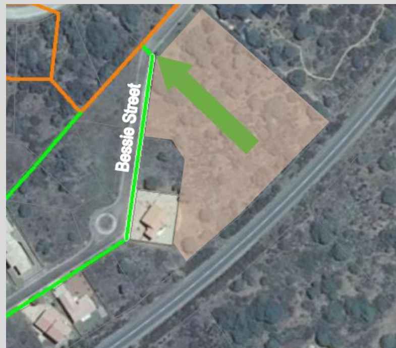
Figure 6: Sewer connection point onto 160mm municipal line (Element Engineers).
