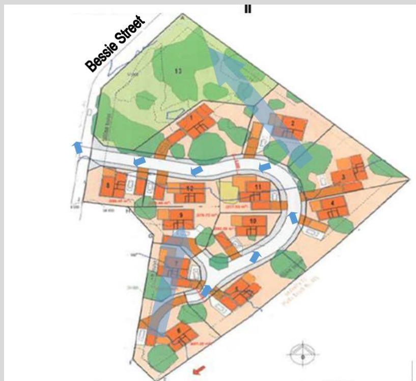
Figure 8: Direction of internal stormwater flow and direction indicated with blue arrows (Element Engineers).
