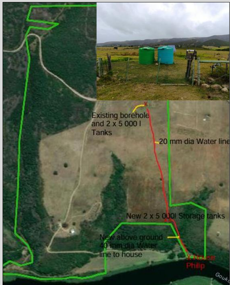
Figure 8: Planned water supply.
