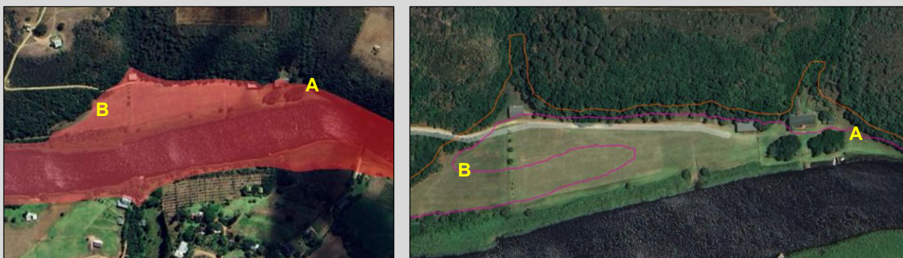
Figure 37: Left: water surface level for the Present 1 in 100 year flood line (WML Coast) at both localities. Right: Coastal Management Lines (red: Coastal Protection Zone; pink: Coastal Management Line).
