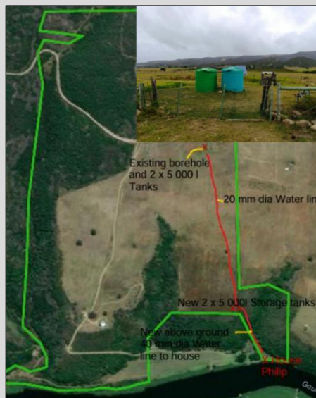
Figure 12: Planned water supply.
