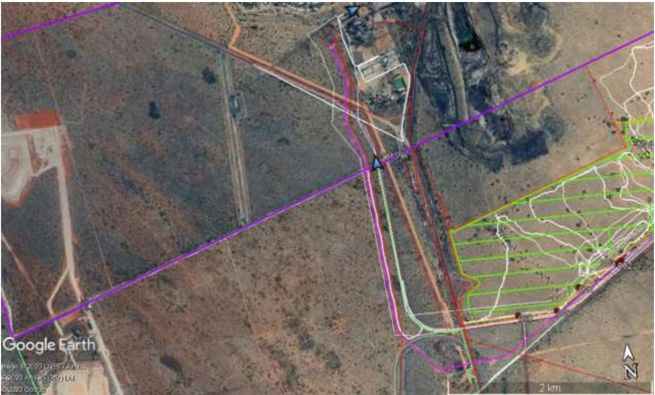
Figure 16: The route of the proposed 132 kV powerline, from the Remaining Extent of farm York A 279, across the railway line and R31, through the property of KMR and Municipal land, connecting with the Hotazel substation, a distance of 6km in total. Our survey tracks are shown in white.
