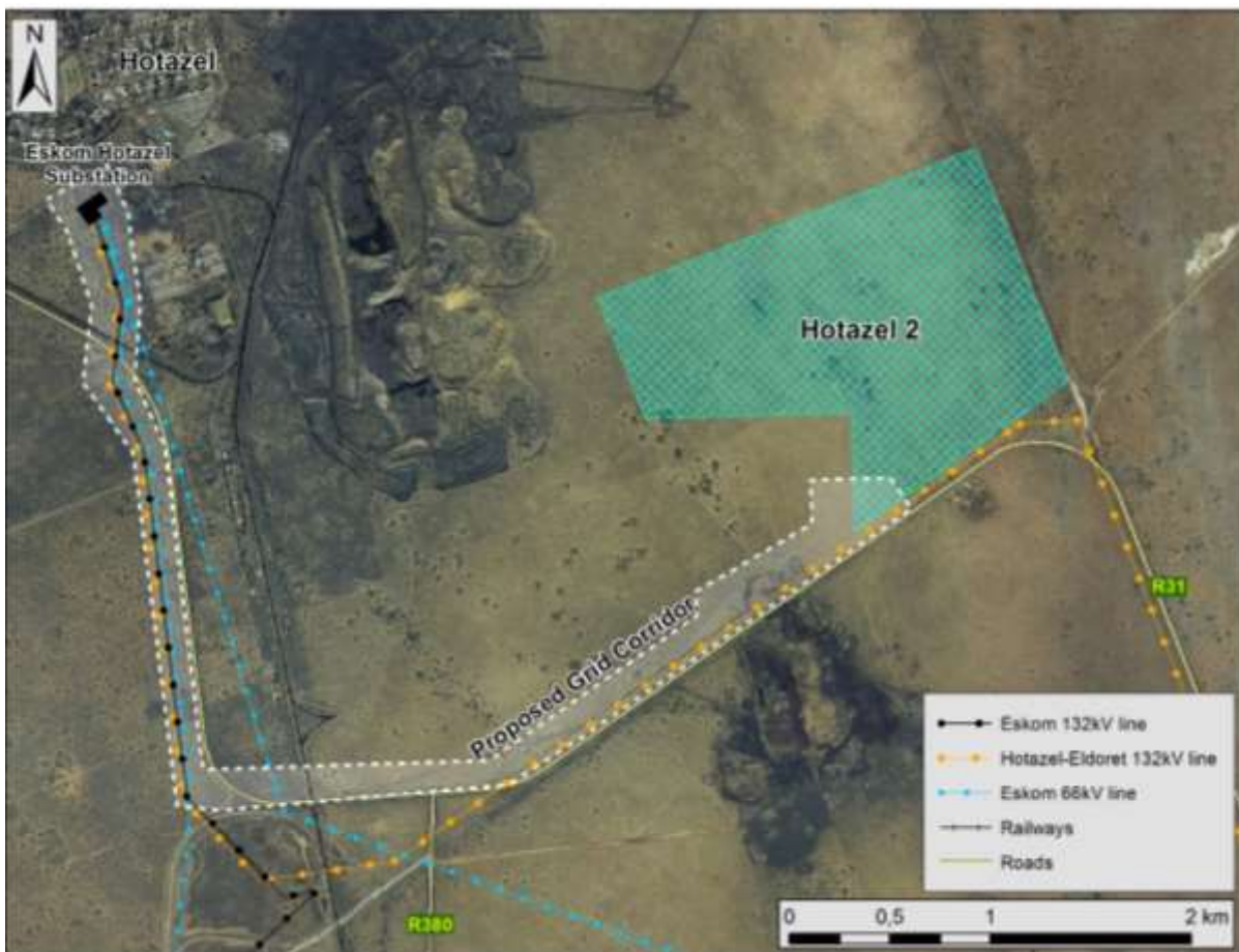
Figure 2: Potential Grid Connection.
