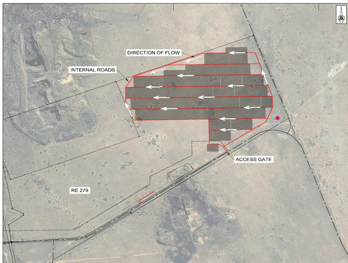
Figure 4.2: Drainage pattern for conceptual layout of PV panels
