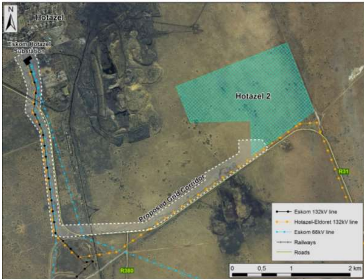
Figure 7: Potential Grid Connection.
