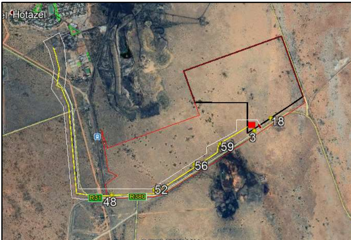
Figure 8: Grid connection (with photo reference points) – The yellow line represents the indicative routing of option 1.
