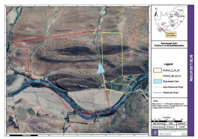
The applicant replaced an existing earth dam that had failed multiple times with a new dam approximately 140m upstream of the previous dam. The new dam storage proposed is  $\pm$ 149 621m<sup>3</sup>. This is to accommodate water from the non-perennial watercourse and to store water from the Buffelsrivier Scheme.
