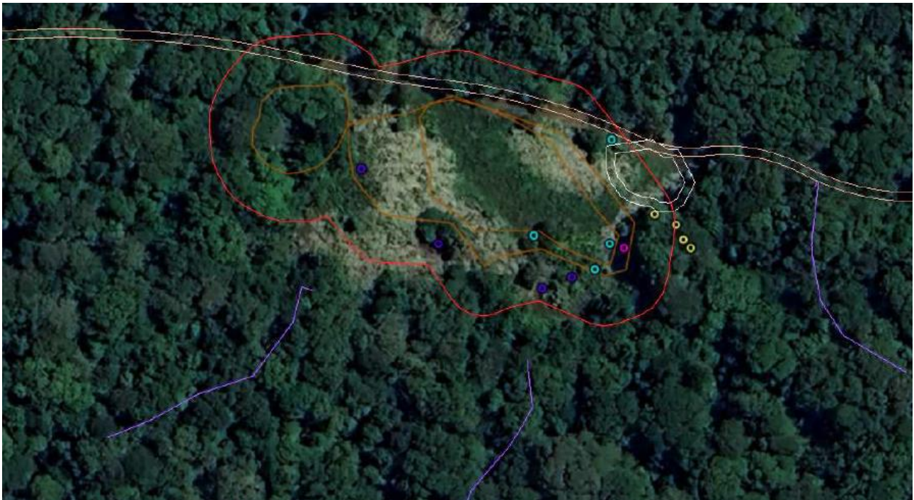
Figure 40: Site sensitivities / constraints identified by the specialists. Coloured dots indicate trees to be avoided, while orange lines indicated pool & wetland with associated 10m (red).
