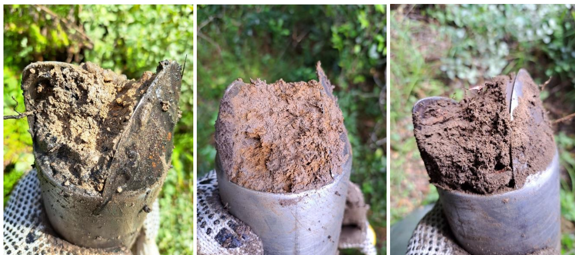
Figure 10. Typical soil auger samples from seasonal (left), temporary (middle) and non-wetland (right) areas of the clearing. All soils are collected within the upper 50 cm of the profile.
