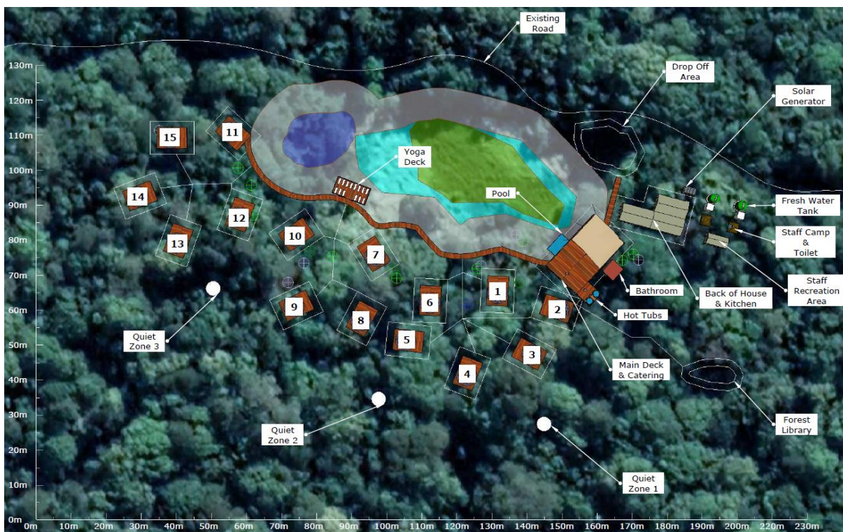
Figure 2: The August 2023 version of the site development plan for the proposed tented camp. One final layout is provided in Appendix 11.5. The dark blue polygon is an excavated pool on the site, the green polygon represents the seasonal wetland with a temporary wetland being the surrounding light blue polygon. The light grey polygon surrounding the pool and wetland areas is the buffer area, as delineated by the aquatic specialist (Dabrowski, 2023).
