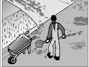
Remove mud from vehicle tyres before leaving site. Care must be taken to place material away from the exit track, in an area where it cannot be washed away. Where possible, do not drive vehicles on and off site during wet weather conditions (i.e. when the site is muddy).
