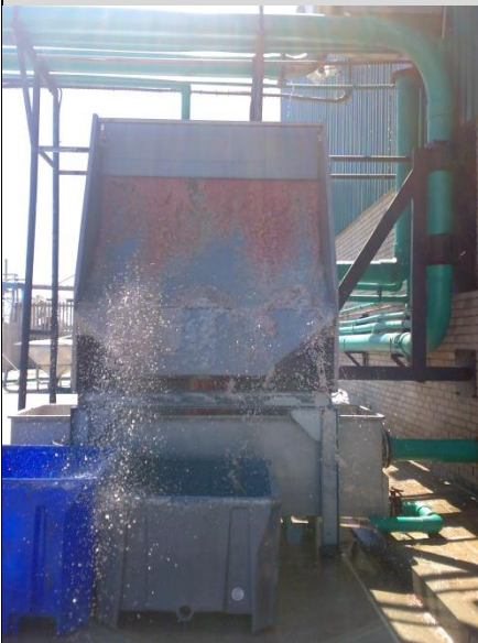
Photo 4: Screen removing solids from the water
