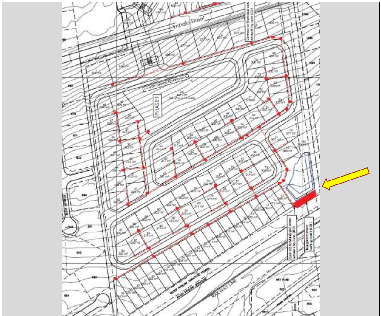
Figure 17: Position of potential 62kl conservancy/holding tank for Phase 1 (Source: Element Engineers).
