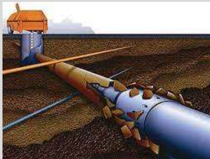
Figure 8: Schematic example of pipe bursting method (Source: https://www.google.com.Fpipespy.com ).
