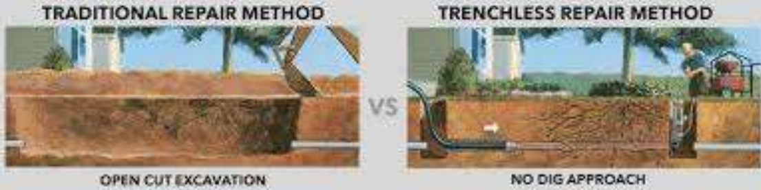
Figure 7: Comparison between standard excavation/traditional upgrade method and trenchless/pipe bursting method (Source: https://www.google.curryandsonsconstruction.com ).
