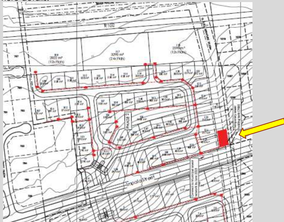
Figure 16: Position for possible 76kl conservancy/holding tank for Phase 2 within Municipal servitude on the property (Source: Element Engineers).
