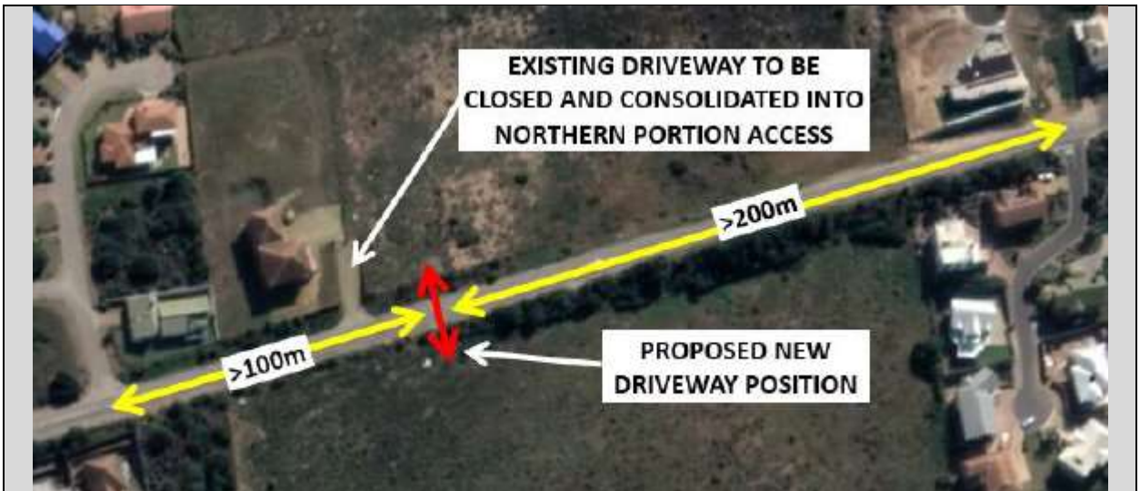
Figure 21: Two dual accesses off Impala Street to the north and southern portions.
