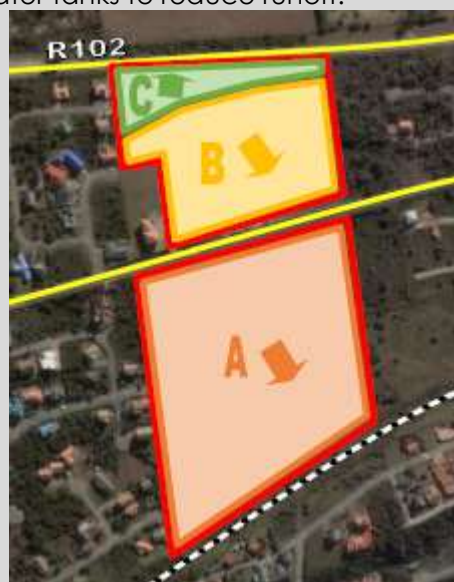
Figure 19: Stormwater drainage catchments for the study site (Source: Element Engineers 2019).
