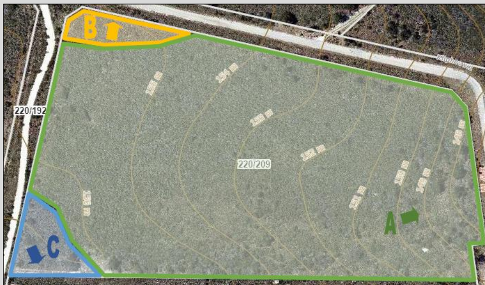
Figure 11: Stormwater Drainage Zones (Stormwater Management Plan, 2024).
