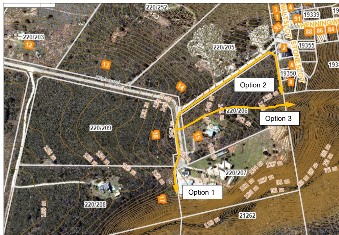
Figure 10: Three external stormwater options on eastern boundary.
