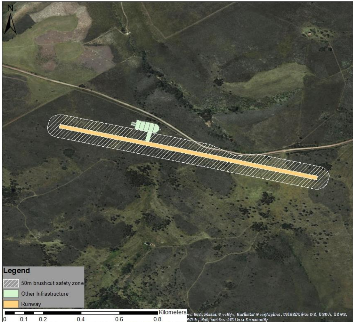
Figure 1.2: Map showing the proposed layout of the airstrip and associated safety zone.
