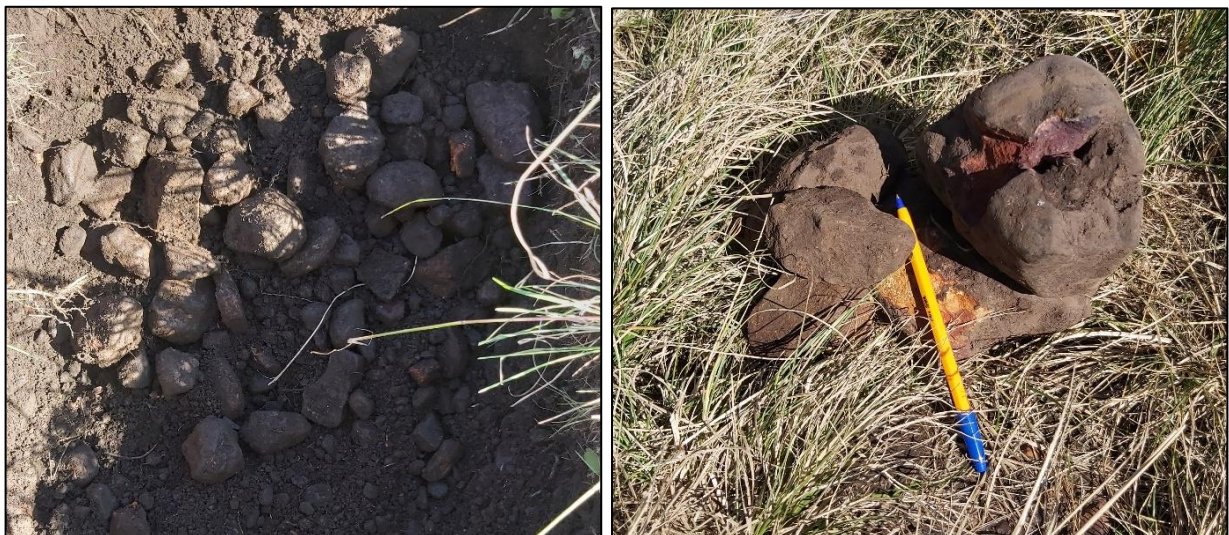
Figure 8: 100 – 400 mm layer consisting of quartzitic pebbles, cobbles & boulders.
