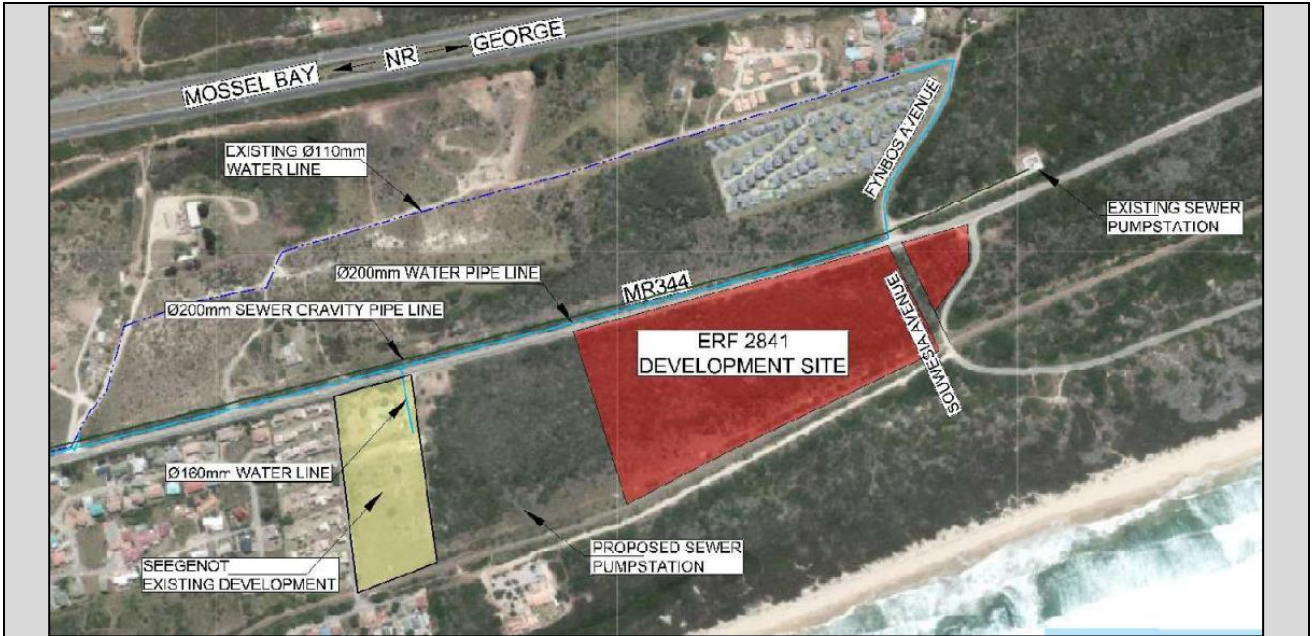
Figure 4: Existing services in proximity to Remainder of Erf 2841 (Extract From Engineering Services Report, 2024).
