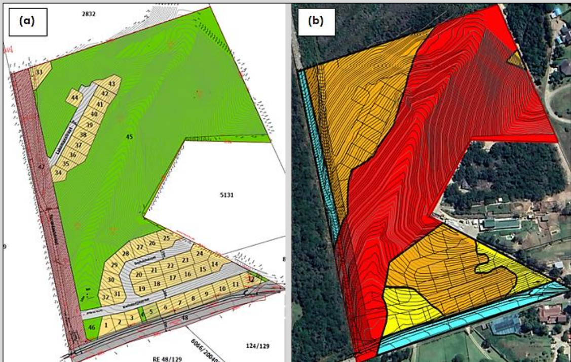
Figure 36: (a) Mitigated Site Development Plan. (b) Mitigated Site Development Plan overlaid onto the Combined Sensitivity Map (Aquatic, Botanical, Biodiversity & Fauna). Development remains within areas identified as having either a medium (orange) or low (yellow) sensitivity. Development within the highly sensitive thicket valley (red) will be avoided leaving +/- 60% of the site undeveloped.
