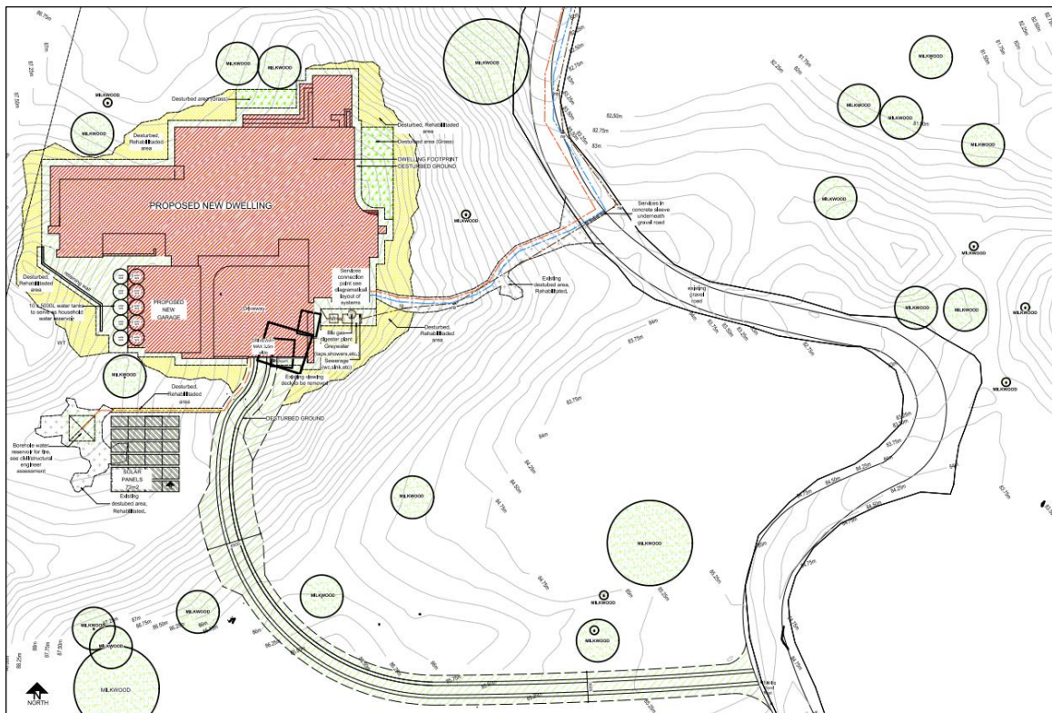
Figure 2: Detailed site layout plan of the Preferred Design Alternative (source: Konka Studio).
