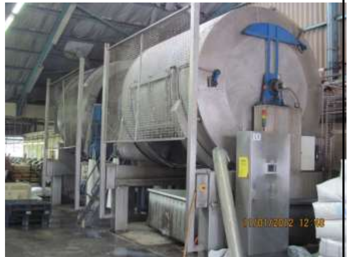
Figure 2: Showing mechanical enclosed drums where pre-tanning and tanning takes place.
