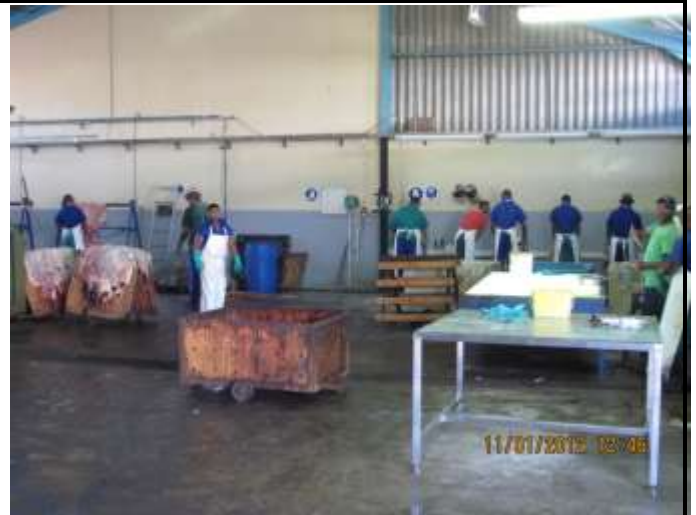
Figure 1: Showing skin receiving area where excess flesh is removed and skins are trimmed, salted and stored.
