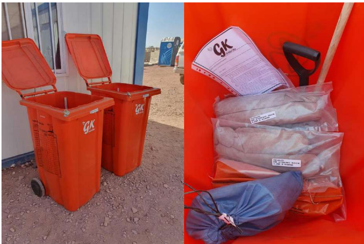
Figure 20: Hydrocarbon Spill Kits must be in place within the site camp, at each work area and in the field within 500m of any drilling or ramming activity.
