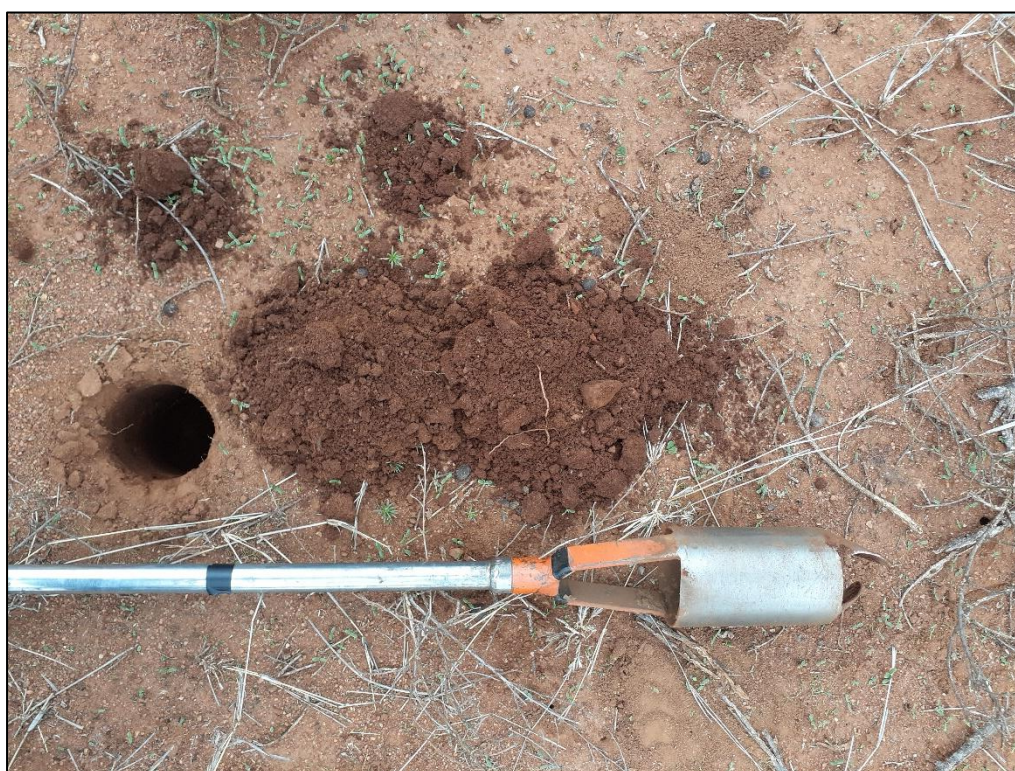
Figure 9: Shallow Mispah profile of 250mm deep at survey point 115
