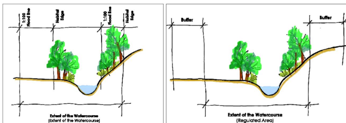
Figure 3-12 Illustration of the extent of a watercourse and the Regulated Area (DWA, 2012)
