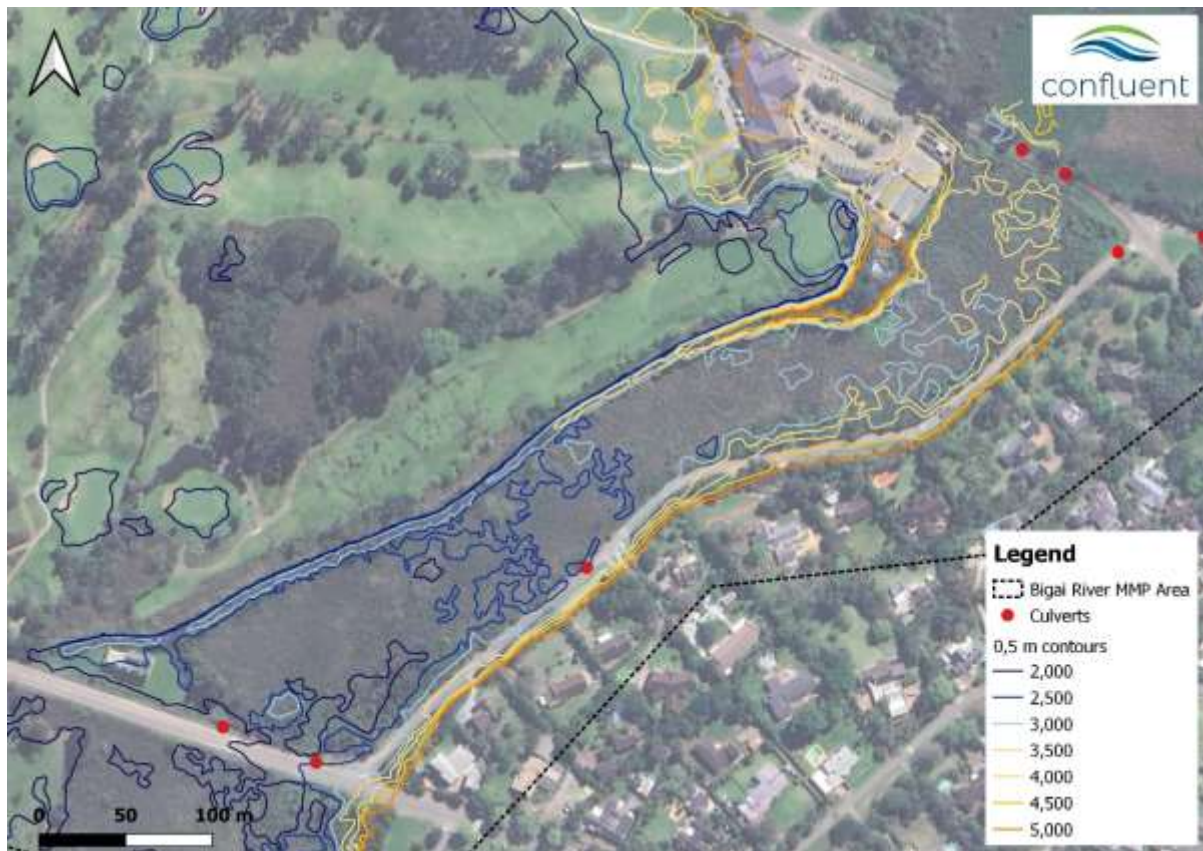
Figure 8. Contours of the Bigai River between Howard Street and Wilson Street in relation to culverts. Based on 2013 Lidar survey of coastal areas (DEA&DP).
