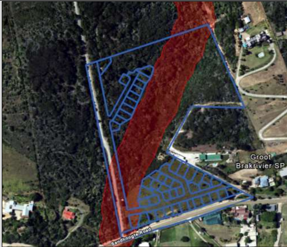
Figure 25: Mitigated SDP showing that all erven are outside the 30m buffer as recommended by Dr Dabrowski.
