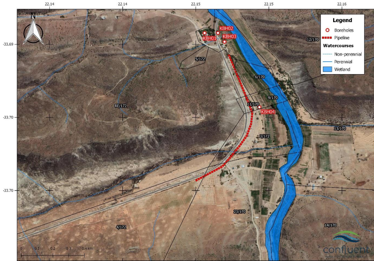
Figure 2: Position of boreholes and pipeline for transferring water to Portion 4 of Farm 172.
