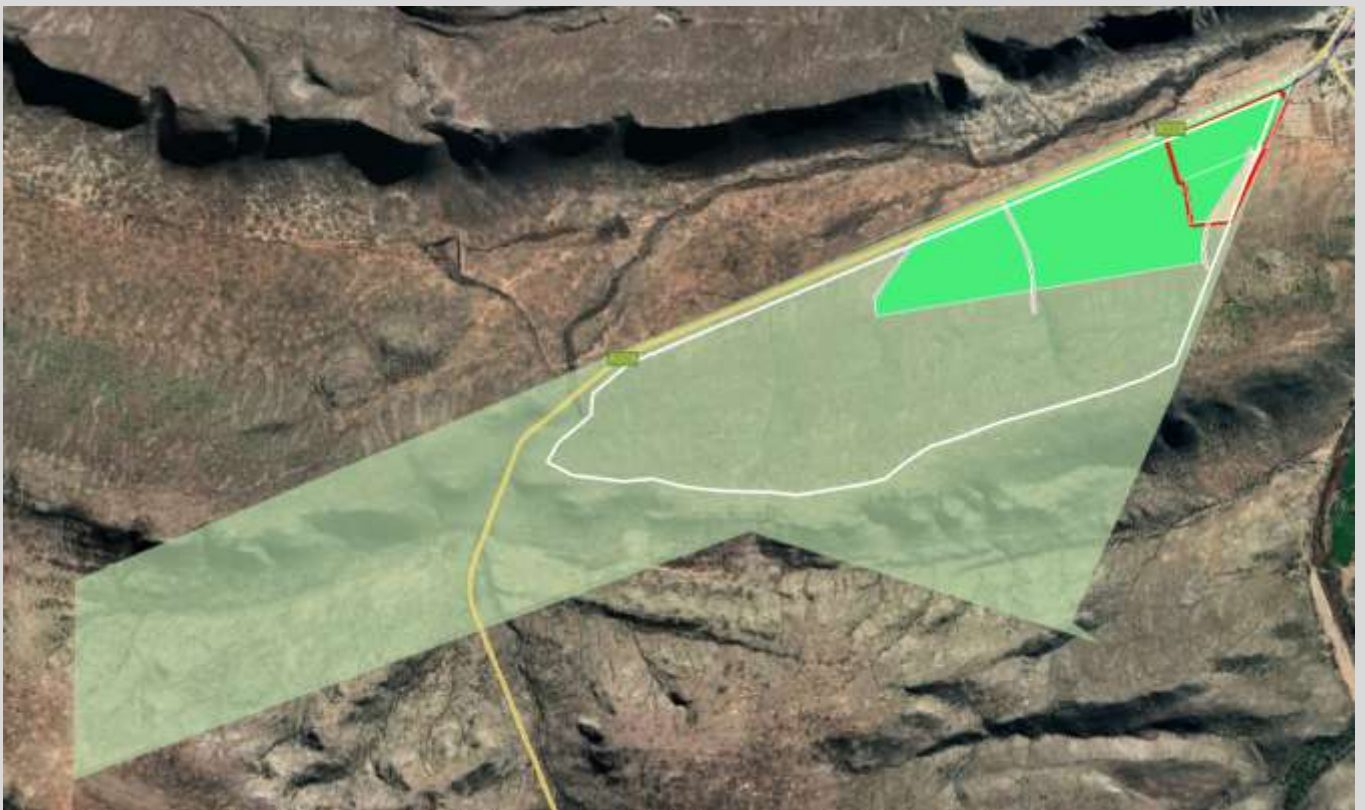
Figure 8: Schematic indication of the original extent planned for 70ha (indicated with white polygon) compared to the reduced 56ha (bright green) and the 13ha already transformed (indicated with red polygon).
