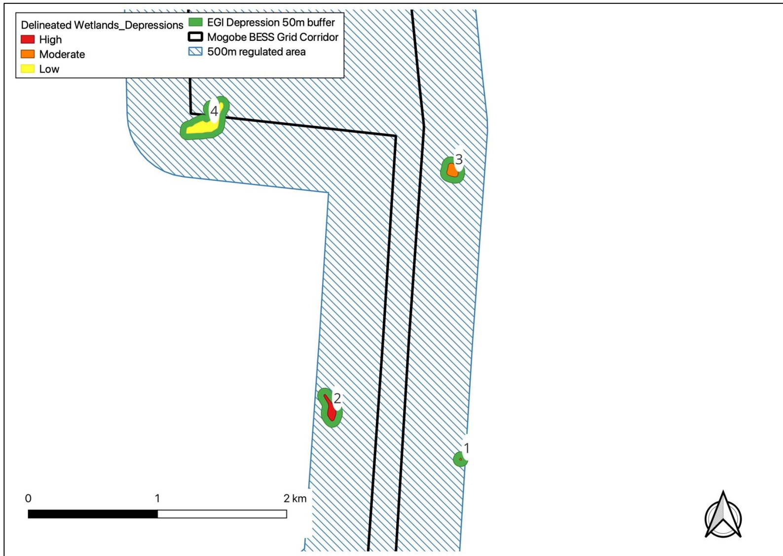
Figure 5: Overall sensitivity rating for the various aquatic systems. Note the 50m no-go buffer is also indicated.
