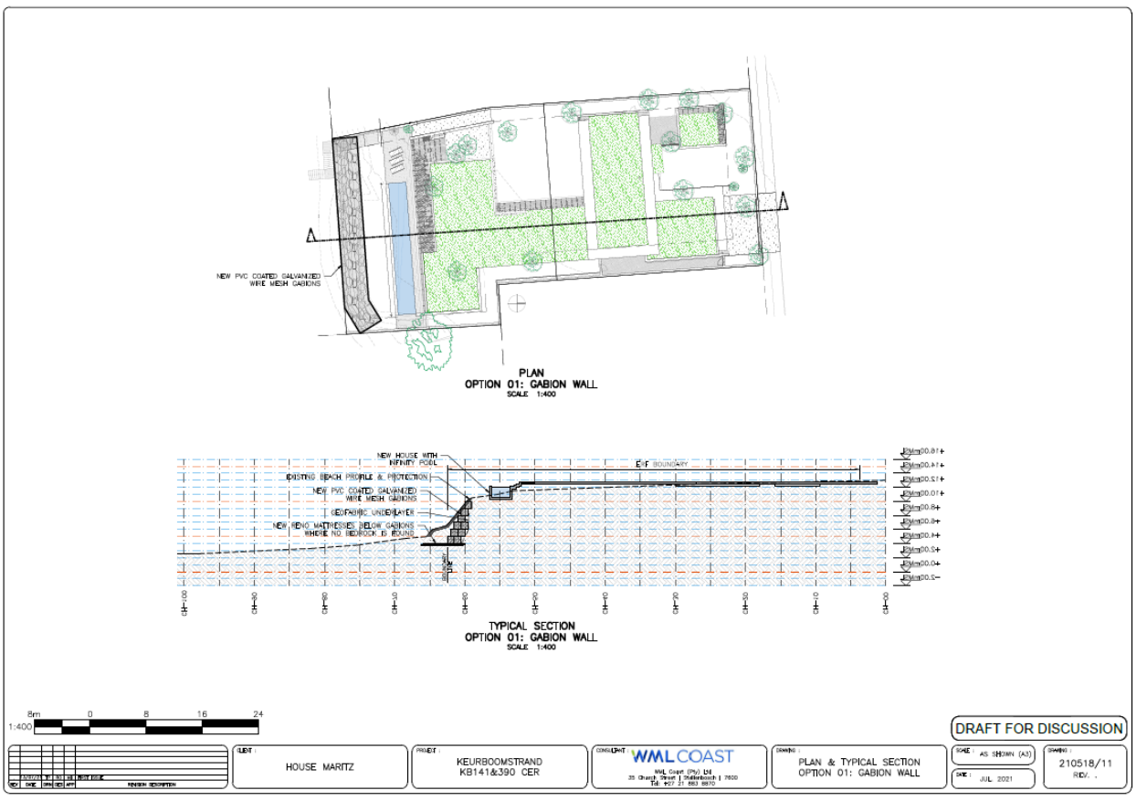
Figure 16: Alternative 1-OPTION 01: GABION WALL
